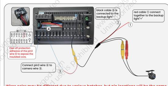
Wires color may be different due to various batches, but pin locations will be the same.
