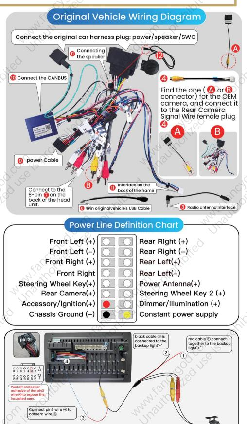
Wires color may be different due to various batches, but pin locations will be the same.
