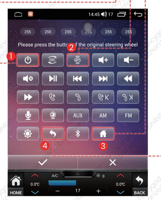
Please first press and hold one of the buttons on the dash kit, then press the related button on the "Control" app interface to learn its feature; learn all buttons one by one accordingly and then click "\sqrt{"} to save the learning process.
