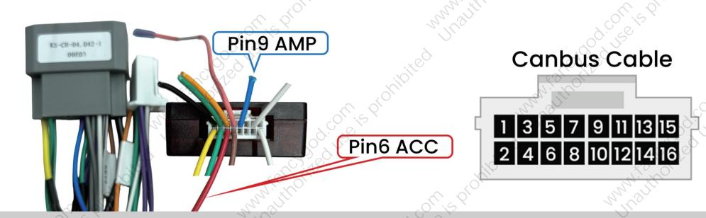
If there is no sound after installation, please manually connect the AMP cable to the ACC cable (refer to pic 1), ensure the connection is correcet in order to power on the AMP and make the sound work.
