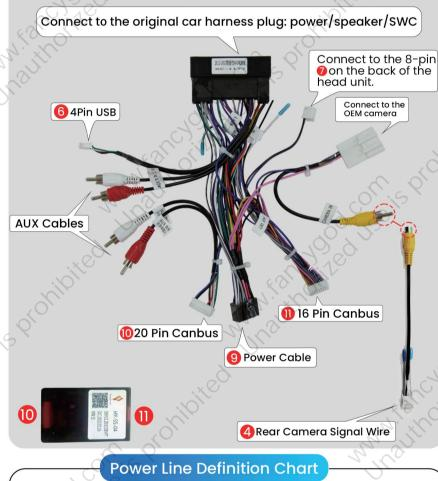
Original Vehicle Wiring Diagram
