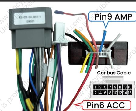
If there is no sound after installation, please manually connect the AMP cable to the ACC cable (refer to pic 2), ensure the connection is correcet in order to power on the AMP and make the sound work.
