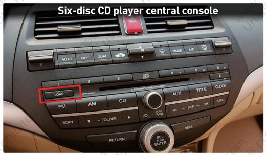
Sound issues: Please use the appropriate harness according to the type of the original CD. Then press the "AUX" button on the original car's control panel for the audio to play from the radio.
