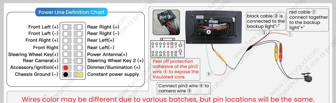
Note: please select the correct wiring harness (A-cables or B-cables) according to the shape and pin configuration of the factory car's plug.
