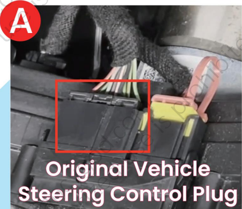
Remove the original vehicle steering control plug
